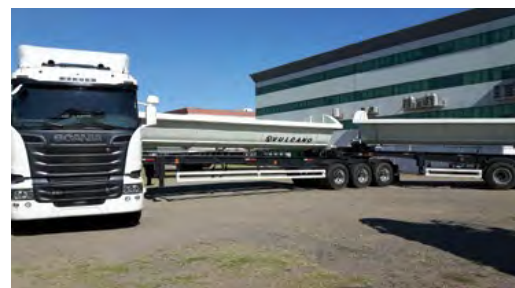
A “Bitren”, double-articulated vehicle for high-efficiency long-distance transport of aggregates, now used in Mexico and Argentina
